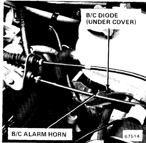
Figure 4 - Ahead Of Coolant Reservoir
