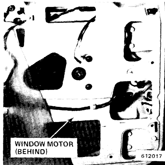
Figure 4 - Inside Driver's Door
